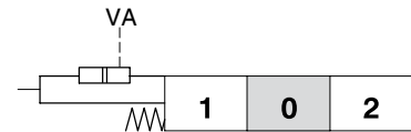
8I11 type With external hydraulic pilot to return from position 1 to neutral
